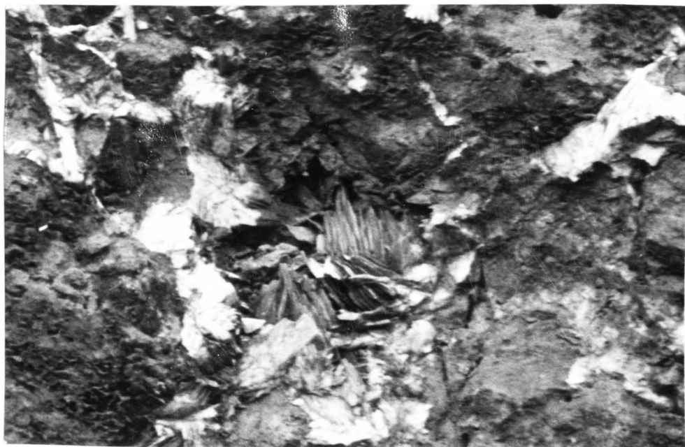
Figures 16a, 16 b - Bladed crystals of barite in the outcrop on the Hornsey Brothers Mining Company, southwest of Potosi (Section out of Figures 2 and 3). One crystal cavity showing centripetal growth of barite is seen in the marked area on Figure 16a and is enlarged on Figure 16b.
